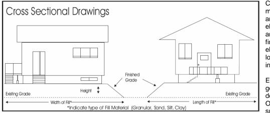
Cross sections must show existing and final grade elevations, existing and proposed finished floor elevations, and lowest openings into buildings.
